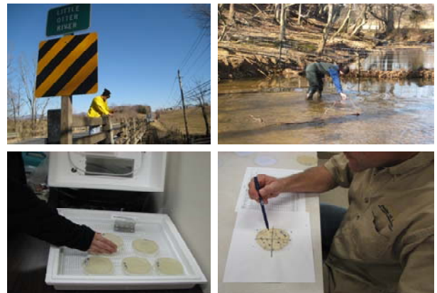
Bacterial water monitoring is conducted monthly by the District using the Coliscan Easygel method.
